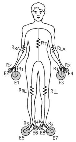
**Figure 1** Measurement pathways of InBody 3.0 (reproduced with permission from Biospace). The subject stands with her or his soles in contact with the foot electrodes and grabs the hand electrodes. Abbreviations:  $R_{RA}$  = resistance of right arm;  $R_{T}$  = resistance of trunk;  $R_{LA}$  = resistance of left arm;  $R_{RL}$  = resistance of right leg;  $R_{LL}$  = resistance of left leg (see text for details).
